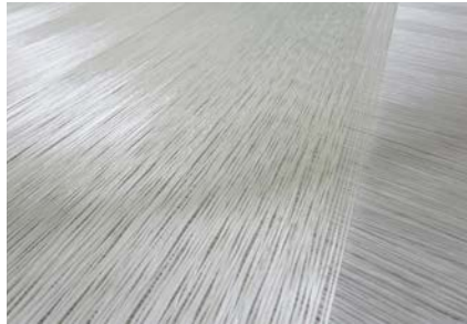
Treated C/E-glass fiber yarn
