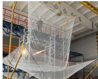
Horizontal debris net construction.
