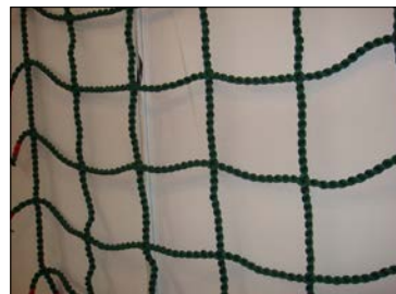
Unknotted horizontal debris netting.
